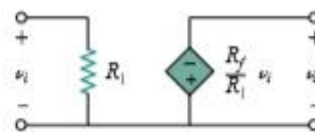
Figure 5.11 An equivalent circuit for the inverter in Fig. 5.10.
